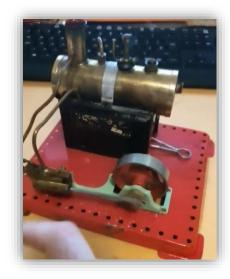
At home, I've put together this Mamod Steam engine which sits on my desk at home. It heats up tap water in the boiler with a special type of candle underneath, then the steam pushes a piston to turn a flywheel. I've also been learning some 3D design software so I can begin to bring my robots and things to life. I put together this Mamod Steam engine model, then made a 3D model of it which I'm going to then animate.
